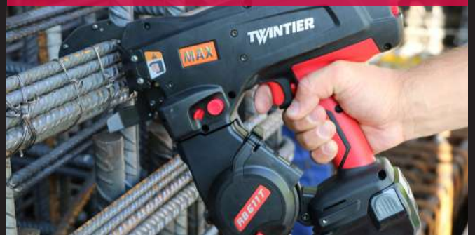
Multiple rebar tying
