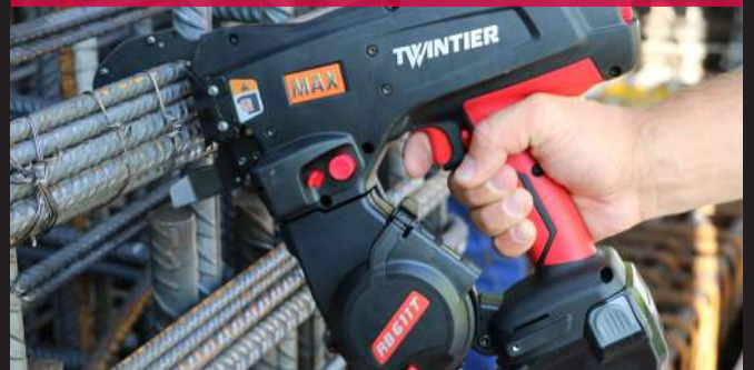
Multiple rebar tying
